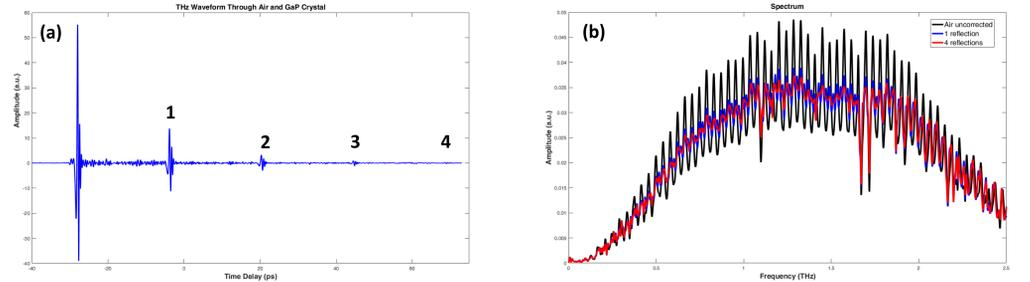
Figure 4: a) Time trace of a 4 reflection THz pulse through N<sub>2</sub> purged air. b) Removal of GaP reflections in the spectrum. Water absorption lines at 1.1 and 1.7 THz are preserved.
