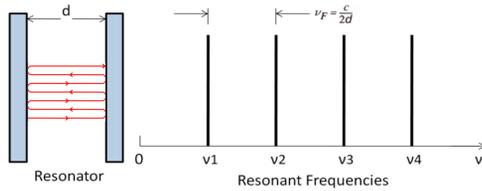
Figure 1: Optical Etalon produces resonant frequencies with a characteristic spacing
